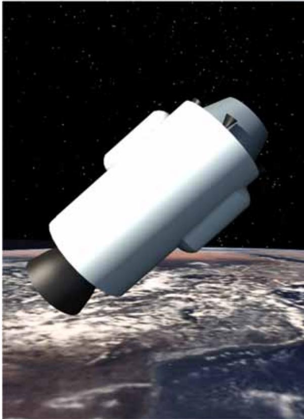
**Phase 1. Development of autonomous on-board de-orbiting system (ADS) for separate orbital stages of SLV based on gasification of unspent propellant components and usage of this power resource for de-orbiting maneuver.**
