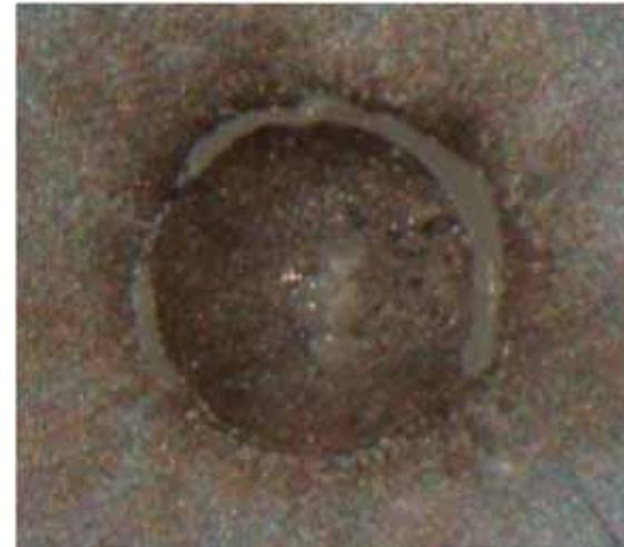
Appearance after launching on a Al flyer target deposited by ion beam sputtering
