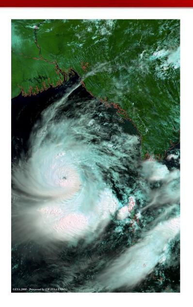
**Envisat captures Cyclone** Nargis making its way across the Bay of Bengal just south of Myanmar on 1 May 2008, with its Medium Resolution **Imaging Spectrometer** (MERIS) instrument working in Reduced Resolution mode to deliver a spatial resolution of 1200 metres.
