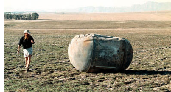
Recovered Delta second stage propellant tank
