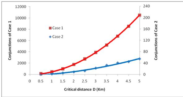
Fig.2 Cumulative distribution of conjunctions as function of critical distance
