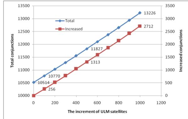
Fig.3 : Conjunction numbers with growth of ULM satellites
