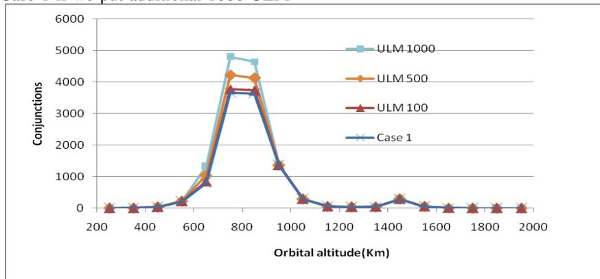
Fig.4: Comparison of altitude distributions of four different scenarios. From top to bottom: 1000 ULM satellites growth, 500 ULM satellites growth, 100 ULM satellites growth, case 1.
