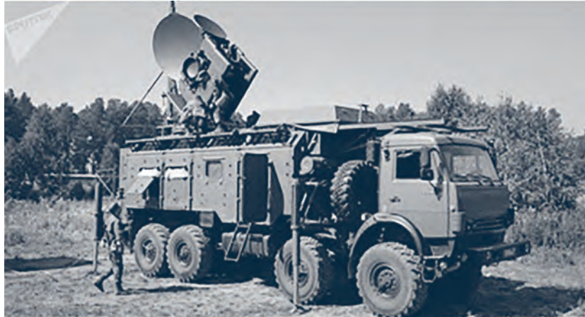
A Russian mobile electronic warfare system used to jam radar. Image credit: Sputnik News. 241
