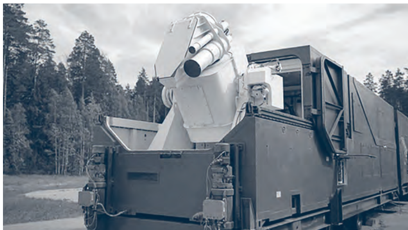
A Russian mobile laser system used to dazzle aerial and space reconnaissance assets. Image credit: Russian Ministry of Defense 262
