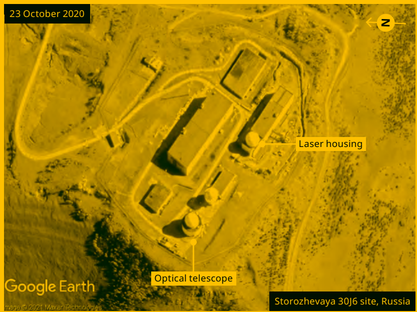
FIGURE 16-49 – KRONA 30J6 OPTICAL COMPLEX NEAR STOROZHEVAYA
