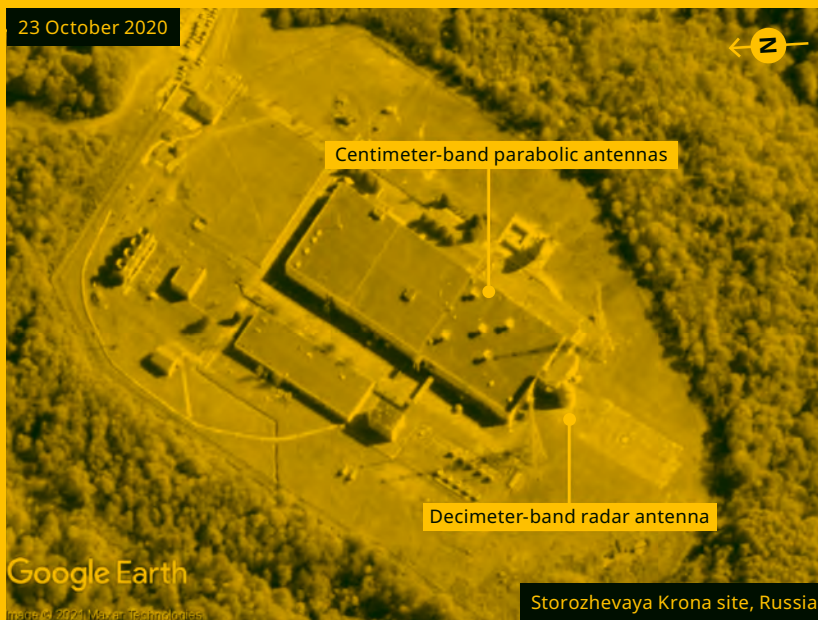
FIGURE 16-48 – KRONA RADAR COMPLEX NEAR STOROZHEVAYA
