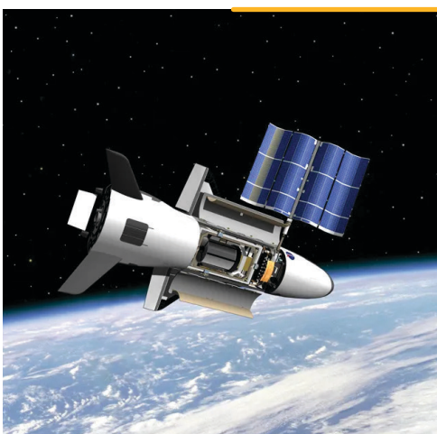
Artist's rendition of how the X-37B will deploy on orbit, including the solar panels used for electrical power.
