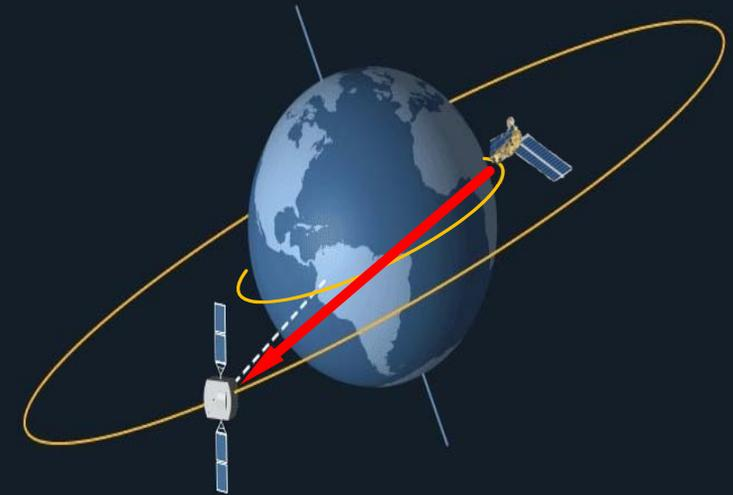
A single sensor satellite tracking a GEO bird from an equatorial LEO orbit. A constellation of these sensor satellites can accurately and continuously scan the entire GEO band.
