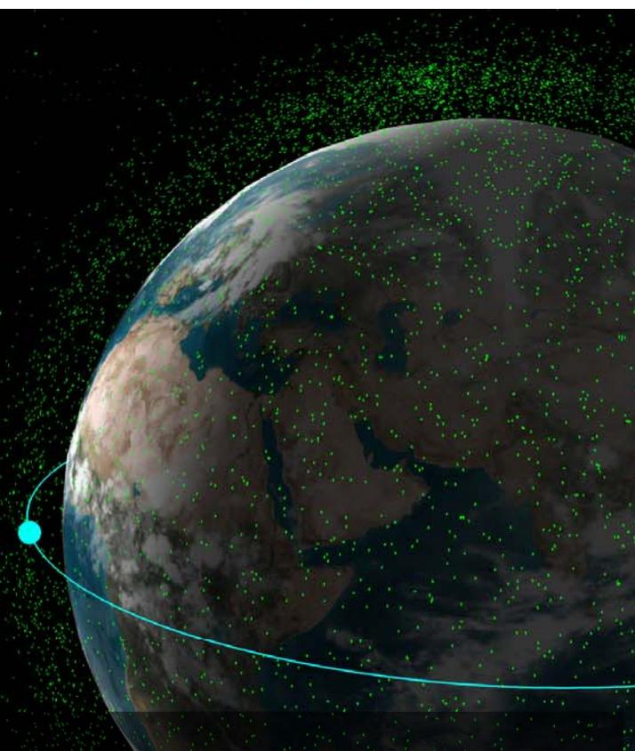
A single debris collector orbits about the equator while it performs in-plane maneuvers allowing small debris to impact its collector pads and avoiding objects large enough to be tracked.
