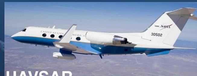
**UAVSAR** Uninhabited Aerial Vehicle Synthetic Aperture Radar
