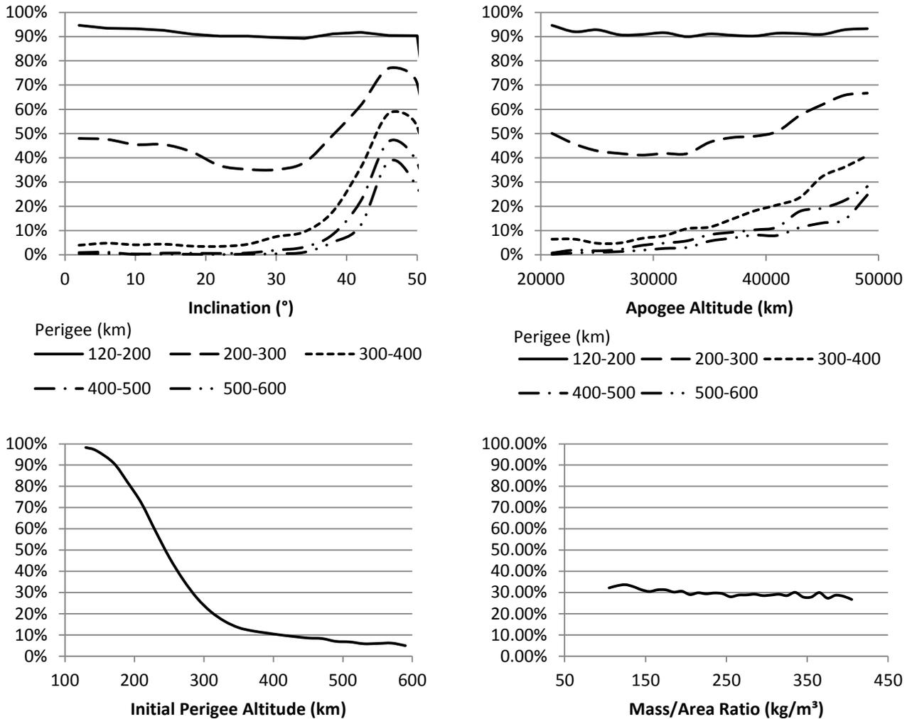
Fig. 5: Probability of debris decay within 25 years for various initial orbital and physical parameters.
