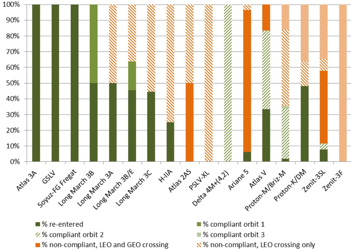
Fig 4: Orbits of upper stages and mission related debris from GEO launches 2004-2012: Launcher breakdown
