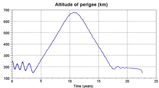
Fig 3: Example of sun-synchronous resonance [4]
