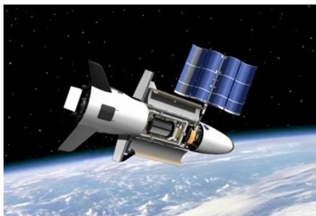
Artist's rendition of how the X-37B will deploy on orbit, including the solar panels used for electrical power. Image credit: Boeing
