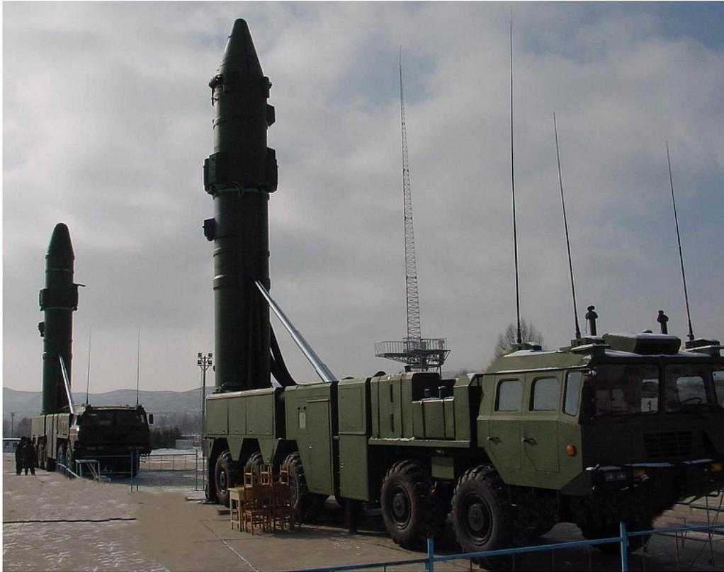
**Figure 9. DF-21C TEL elevated for launch. (Image credit [Air Power Australia](#))**
