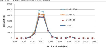
Fig.4: Comparison of altitude distributions of four different scenarios. From top to bottom: 1000 ULM satellites growth, 500 ULM satellites growth, 100 ULM satellites growth, case 1.
