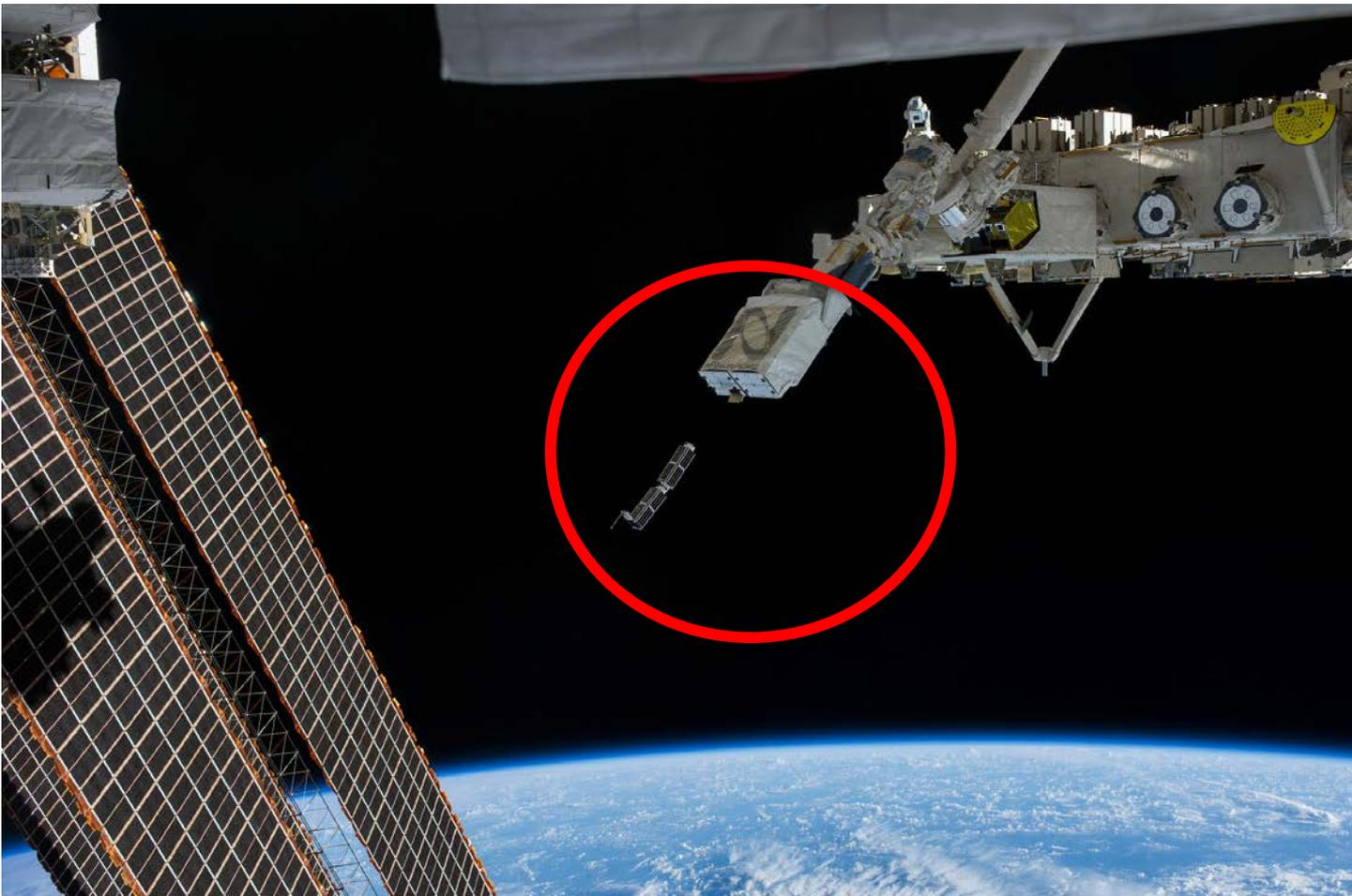
Deployment of PlanetLabs 3U cubesats from NanoRacks deployer on ISS
