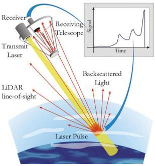
**Figure 5-15:** LiDAR emits laser pulses towards the atmosphere and retrieves frequency of backscatter from clouds, aerosols, and molecules in the atmosphere [ESA, 2008b].
