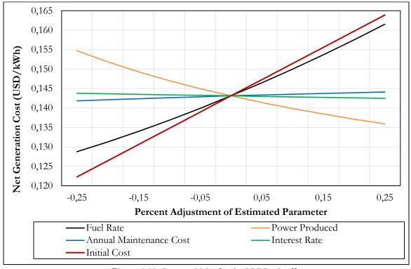
Figure 4-14: Cost sensitivity for the SOFC spinoff.
