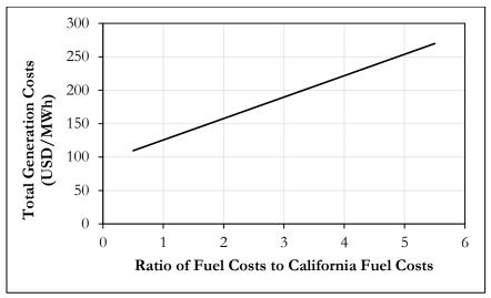
Figure 4-15: SOFC-generated electricity costs as a function of ratio to California fuel prices.
