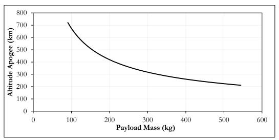
Figure 6-9: Launching characteristics of the Terrier-Malemute sounding rocket [NASA, 2011].
