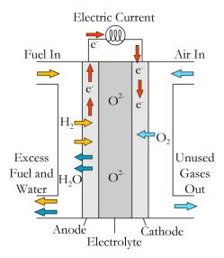
Figure 4-11: Operating principle of an SOFC [Wikimedia Commons, 2007].
