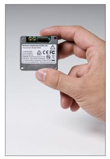
Figure 5-25: Iridium 9602 data transmit modem which could be integrated into collars [Flickr, 2010].
