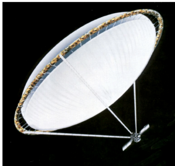
Figure 4-5: Inflatable large solar reflector (Marzwell, JPL)
