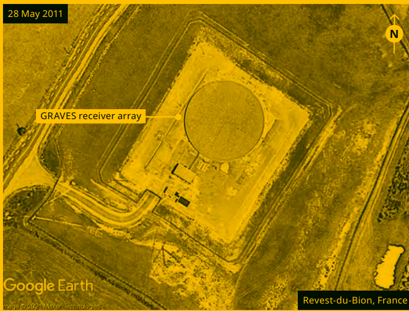
FIGURE 16-54 – GRAVES RADAR RECEIVER
