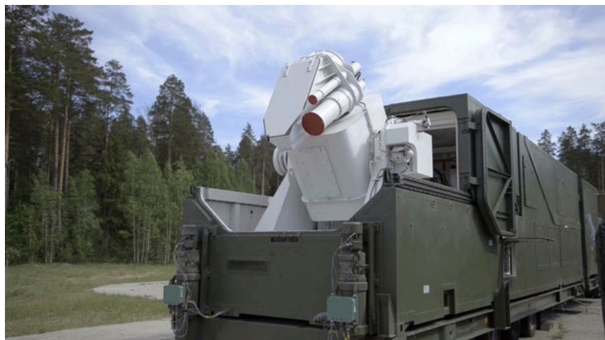
A Russian mobile laser system used to dazzle aerial and space reconnaissance assets. Image credit: Russian Ministry of Defense. 325
